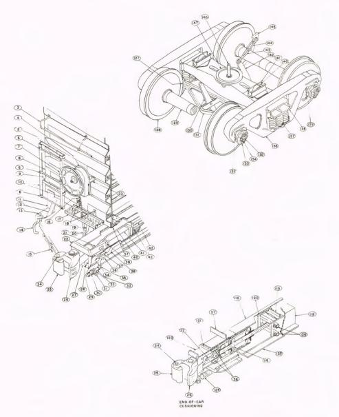
Hand brake housing End ladder support—top End ladder tread 6. 7. Hand brake wheel
