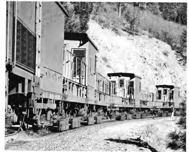
In front of each grinding wheel is a hanging metal strip curtain to keep the metal shavings at track side.
