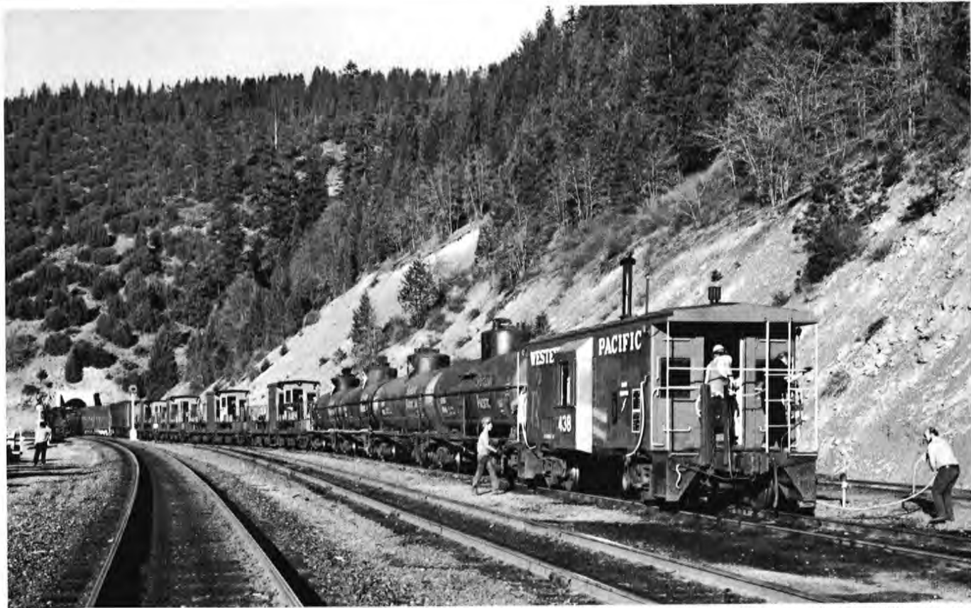
The 11 car rail grinding train switches in to a siding at Keddie at the end of another 12 hour
