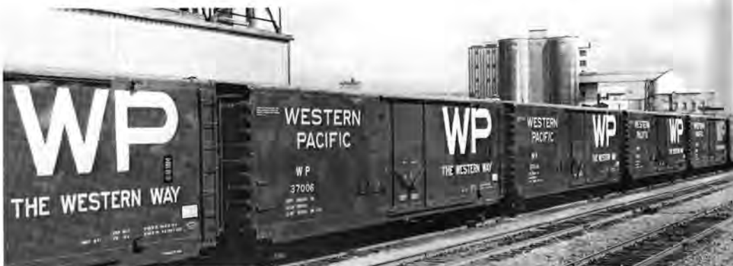
A string of loaded Western Pacific 70-ton, all-steel freight cars built for WP last August. Photo by Don Sims.
