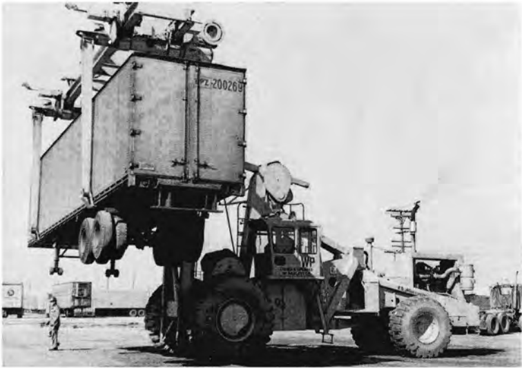
WP's 45-ton capacity LeTourneau side porter easily lifts truck trailer to be carefully set down on rail flatcar. Operator Elim Anderson is assisted by two groundmen, Fred Starling and Robert Abood.
