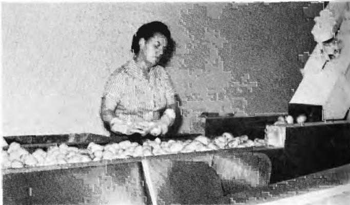
After being peeled by machine at right, any oversized potatoes riding assembly line are sorted and hand-cut by this worker into more uniform size.
