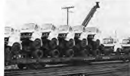
The crew just finished loading pedestal-mounted imported trucks for an experimental load to Maryland. The flat car came in with International Harvester trucks, and WP is using it with their permission in order to get a two-way haul.
