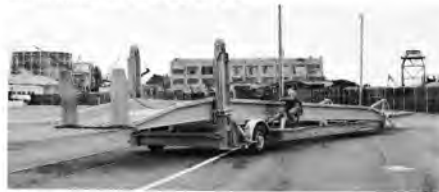
The new self-propelled unloading ramp is portable, easily moved from one track to another, and is driven by one man.
