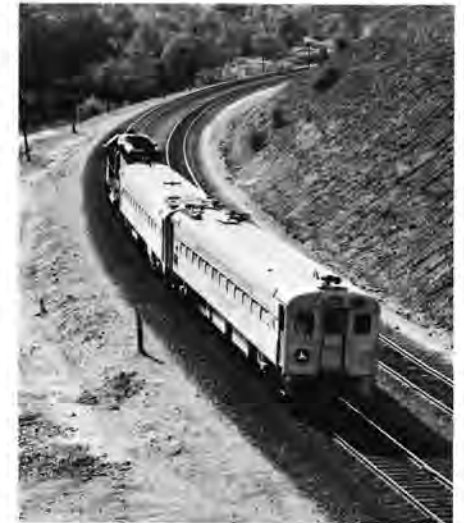
DOT/FRA test cars roll through James during track geometry inspection of the WP main line on November 10, 1977. Photo: Dale Sanders.
