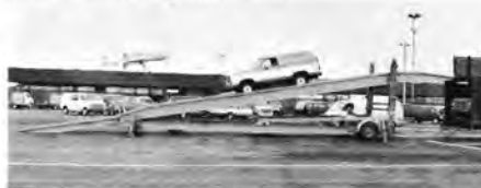
This flexible, new portable "mobile" ramp allows crews to unload cars in almost any area within the distribution center.
