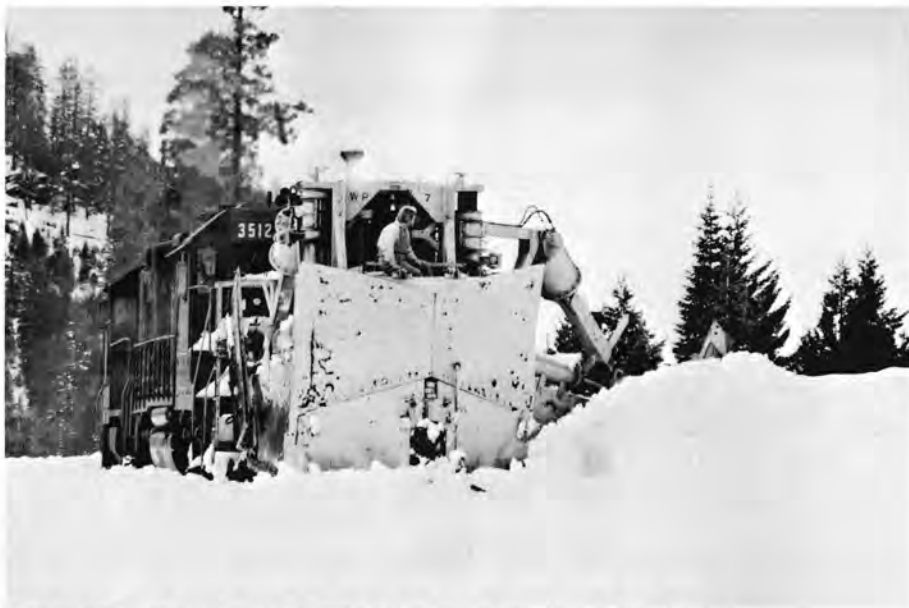
Large steel arms extend from the side of the Jordan Spreader to clear snow from a recent storm. Photo: Dale Sanders.
