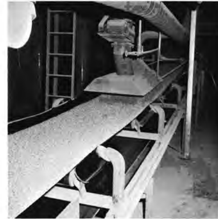
The corn moves through the grain terminal on a series of fast-moving belts.
