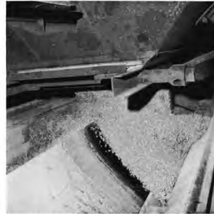
From the dump bins under the covered hoppers the corn moves via conveyors to the top of the grain elevators.
