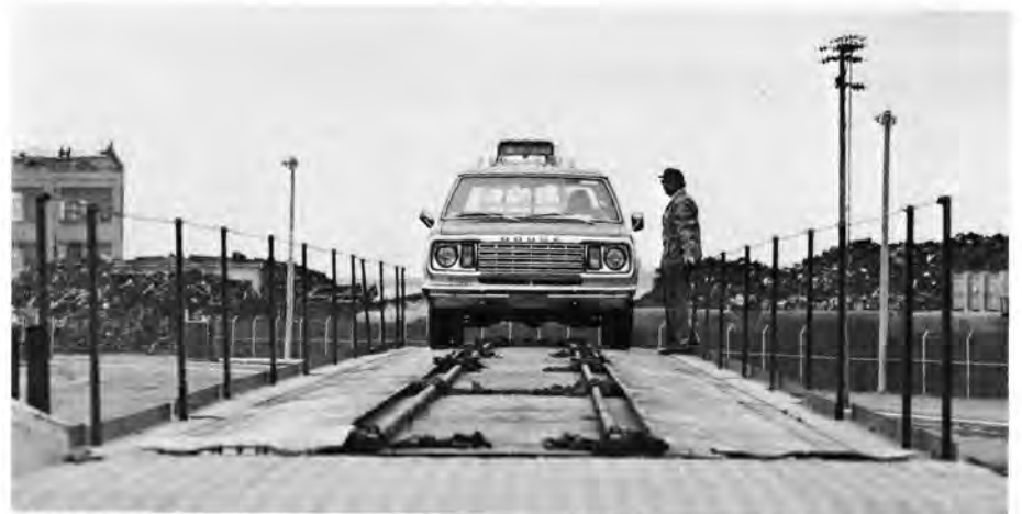
With the "mobile" ramp in place, and tie down chains disconnected, vans and trucks are quickly and easily unloaded. FALL, 1977-8, WINTER
