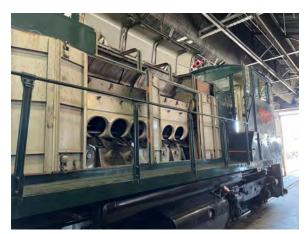
terior of the block, as well as the interior surfaces of the air box. On a two-stroke supercharged diesel engine, the air intake is not just charged for compression, the pressure is also used to clear out the combustion gasses from the power stroke. This process isn't completely smooth, so some of those combustion products end up flowing back into the air box and it makes for quite a mess.
