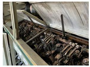
We then removed all the inspection covers in the engine block and opened up the top deck. Inspections were performed on camshaft lobes, rocker arms, valves, injectors, various bolt and nut torque, coolant pipes and connections, piston skirts, piston rings, connecting rods, oil passages, oil lines and various bearings. It was gearhead heaven, at least until it was time to replace all the covers and clean everything again.
