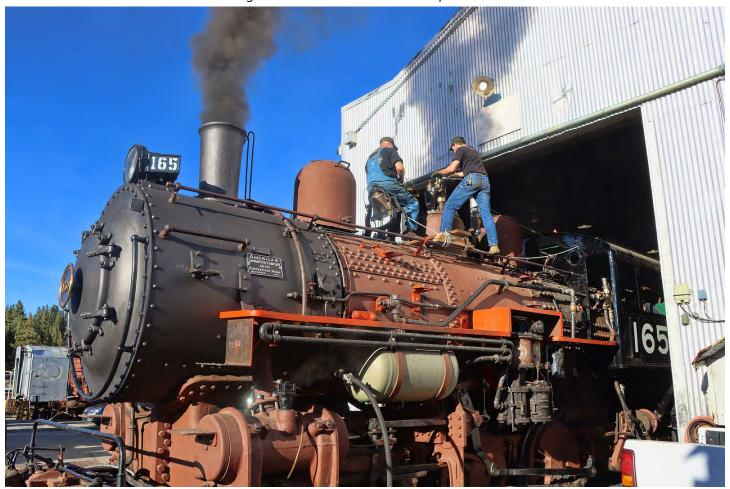
David Elems and Roger Stabler making sure the safety valves are tight before any pressure was raised in the boiler.
