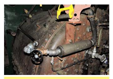
Fireman's Manifold, body manufactured by Channing Walker. Mike and Roger installed it on the engine with the blower valve and associated piping to the smokebox.
