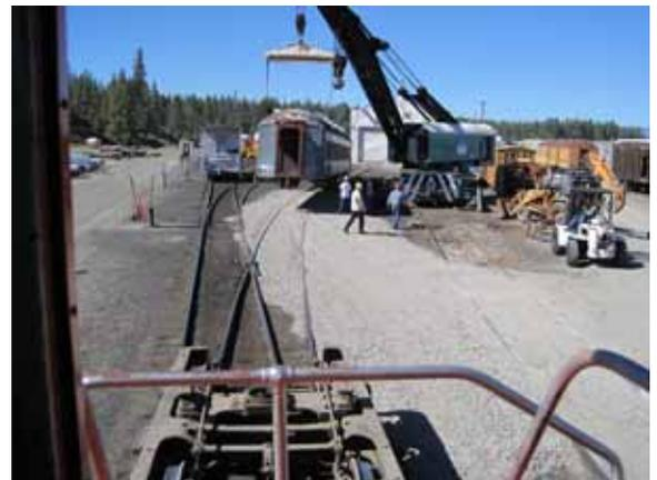
With one end in the air, the crew is ready for the lead trailer to be backed into place. The sub's truck is visible in the foreground through WP 608's handrails.
