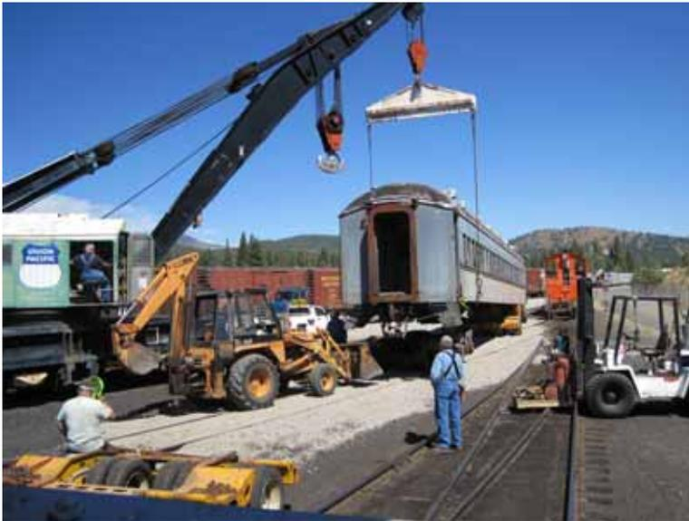
A good overview of just how complicated this could get. As WP derrick MW37 lifts, the backhoe is in place to pull the now released truckset. WP NW2u 608, in the background, pulled the first truckset to allow the lead trailer (the yellow visible under the far end of the car) to be backed into place. The following trailer, in the foreground, will be moved as soon as the truck is away. The big white forklift holds welding gear and other tools at the ready.
