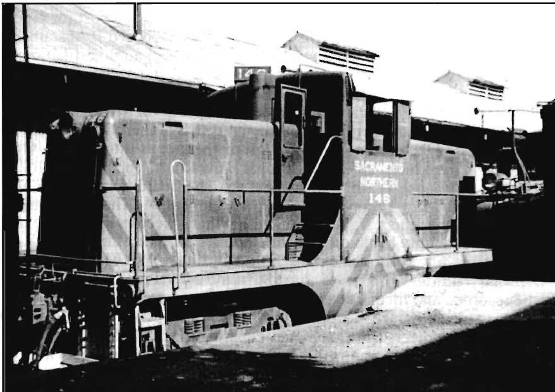
Our SN 146 shows her original paint scheme of black with orange stripes, with silver on portions of the handrails and silver foot boards, while awaiting assignment at Sacramento in the early 1950's. Note the angled number boards on the cab roof but no yellow beacon. SN Steeple Cab #653 is behind her. —Courtesy Brad Lomazzi
