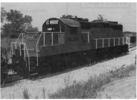
shop, chopped its nose, and changed the control stand to make the unit long-hood forward. The unit was renumbered Relco #2001, the hoods and cab painted in a twotone blue, with black frame and trucks. A few months later, PACIFIC RAIL NEWS reported that RE 2001 was working at an Exxon Chemical plant with RE 1071, an ex-Portland Terminal (Oregon) Alco S-4.
