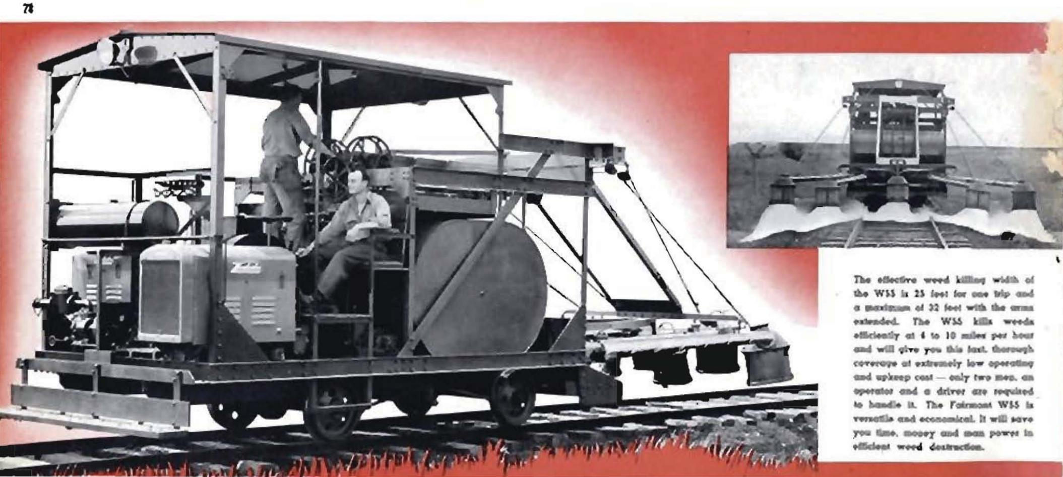
The effective weed killing width of the W55 is 25 feet for one trip and a maximum of 32 feet with the arms extended. The W55 kills weeds efficiently at 4 to 10 miles per hour and will give you this fast, thorough coverage at extremely low operating and upkeep cost — only two men, an operator and a driver are required to handle it. The Fairmont W55 is versatile and economical. It will save you time, money and man power in efficient weed destruction.
