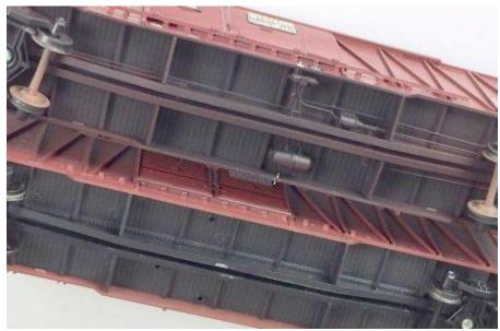
The original MDC underframe is on the lower part of this photo. In comparing the two models, the upgraded car at the top shows the new lower door rail and doors laying on top of the bracing. The AB brake system detail parts are a mix from IM, Tichy and Grandt Line.
