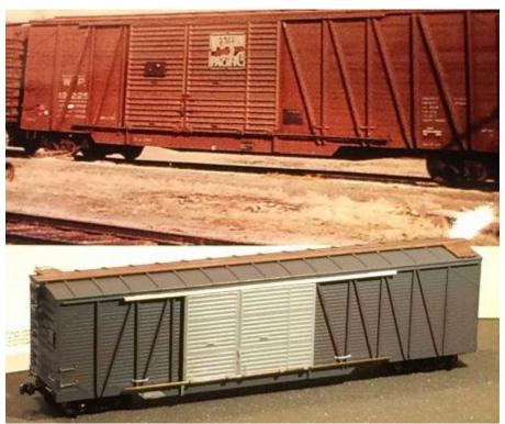
Fred kept prototype images handy to guide the detail work. Note the side sill extension to the left of the doors.
