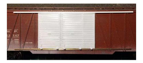
The original doors were replaced with assembled Intermountain 6-foot Youngstown doors. These lay on top of the side bracing. The cast-in rollers were made free standing so they could 'grab' a brass L-profile rail sanded more acceptable proportions. The top rail is a piece of styrene.
