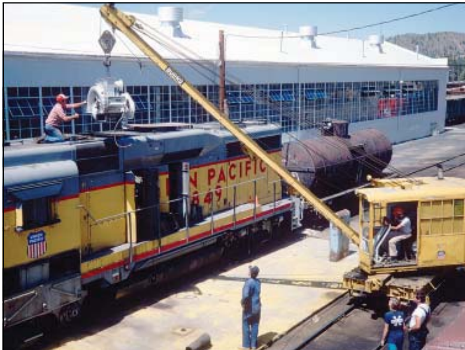
Volunteers spend the day installing a new turbo into UP GP30 849.
