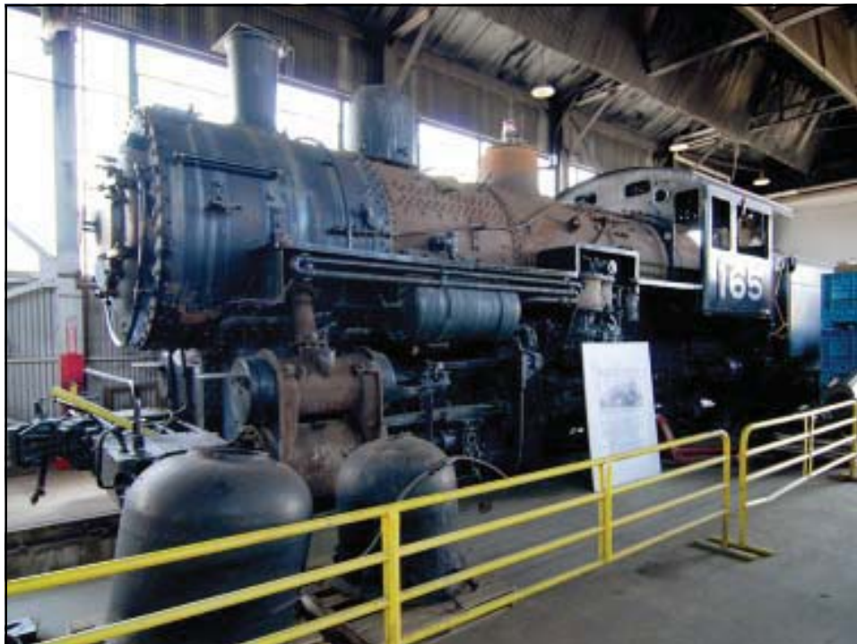
We have a steam locomotive too. WP 165, a 0-6-6 is undergoing a full operational restoration.
