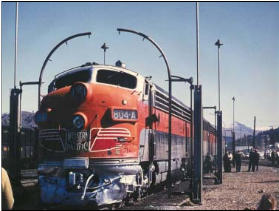
Last westbound CZ enters car washer. Power was not washed as a water-saving policy. Spray was turned on after power passed through.
