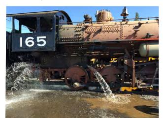
stud holes that we had missed after they were removed. The boiler was washed out in the mud ring and plugs were left out to allow the boiler dry out.
