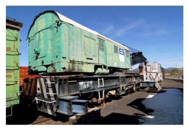
A rear view of the equipment cabin of the MW37. The windows flanking the Union Pacific herald open into the operators cabin, access via a sliding door in the front right corner. The side door leads into the motor area. Originally, the rear section contained a steam boiler.
