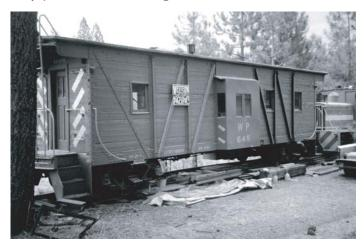
A number of eastern roads had experimented with cabooses that had a bay window on each side instead of a cupola. WP decided to experiment with the construction of a bay window caboose in 1942. Caboose NO. 642 was put into service for evaluation. It was a success and subsequently 60 bay window cabooses were built between 1943 and 1945. Because of the increase in war time traffic the early wooden cabooses remained in service but were mainly used in local service.
