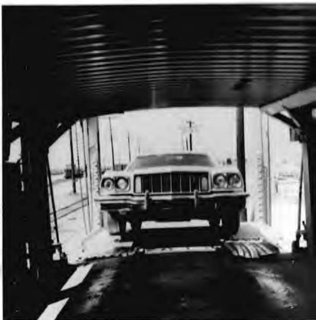
This inside view shows an auto being loaded into the "B" (or second) deck of a tri-level railroad car headed for Jersey City. The loading and tie-down operations can be accomplished in a matter of minutes.
