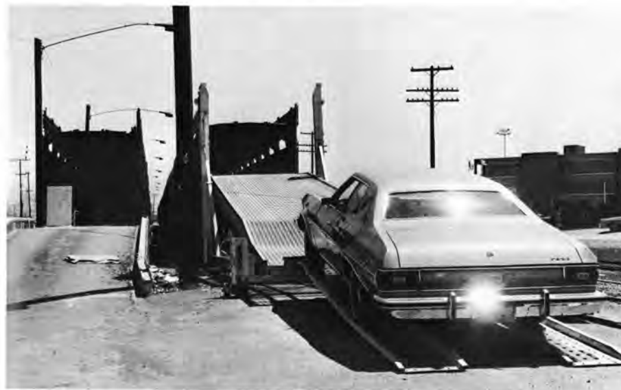
At Western Pacific's Oakland Auto Terminal ramp #1 (right) can handle automobiles on and off of bi-level and tri-level railroad cars,
