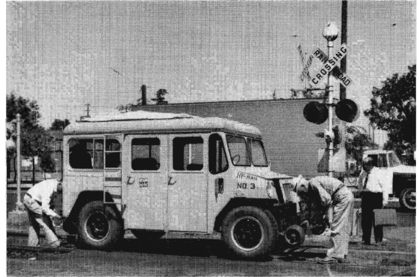
Arriving at Stockton, flanged wheels are raised and Hy-Railer then moved onto City street as an ordinary automobile to refill gas tank at nearby service station. This was done while waiting for meet with westbound California Zephyr.
