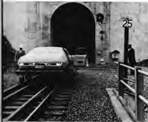
Milepost 231: Track inspection party will pass Milepost 231 inside 8856' Tunnel 8 (longest on railroad) after just crossing 66' Dark Canyon bridge (shortest on relocated main line). Speed limit sign at right.
