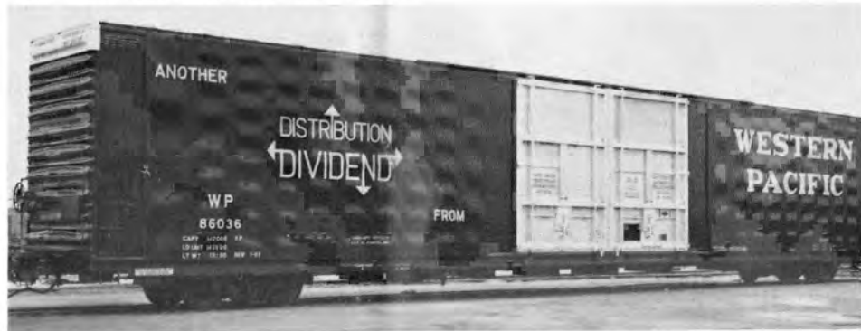
Below: One of W P's 86-foot, high cube, cushion underframe, auto parts cars, with plug-type door for easier loading and unloading.
