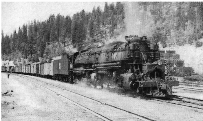
A mighty mountain Mallet sands the rails and with a blast of her twin exhausts commences her 1 per cent climb eastward out of Keddie.
