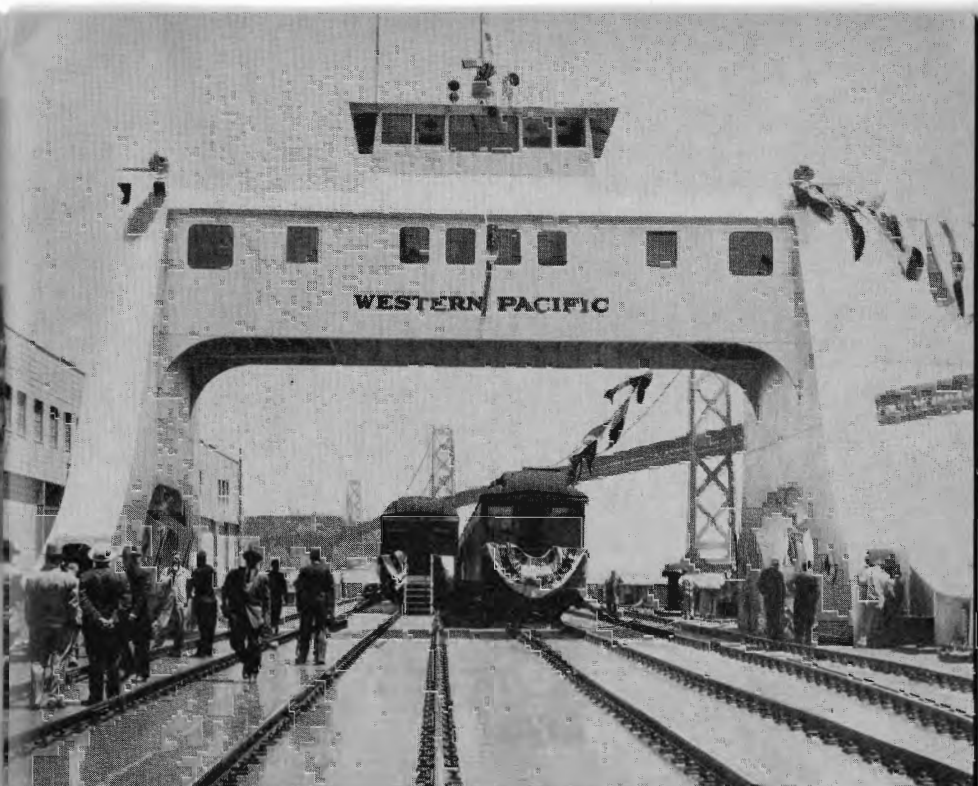
From her deck the vessel's single-span bridge amidship makes an impressive sight. She can handle 28 freight cars on her 375-foot deck.
