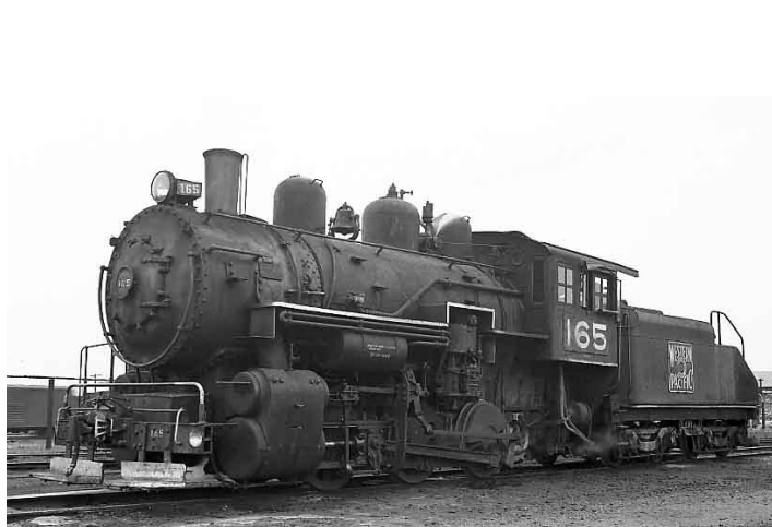
0-6-0 switching locomotive, built Alco-Schenectady, 1919
