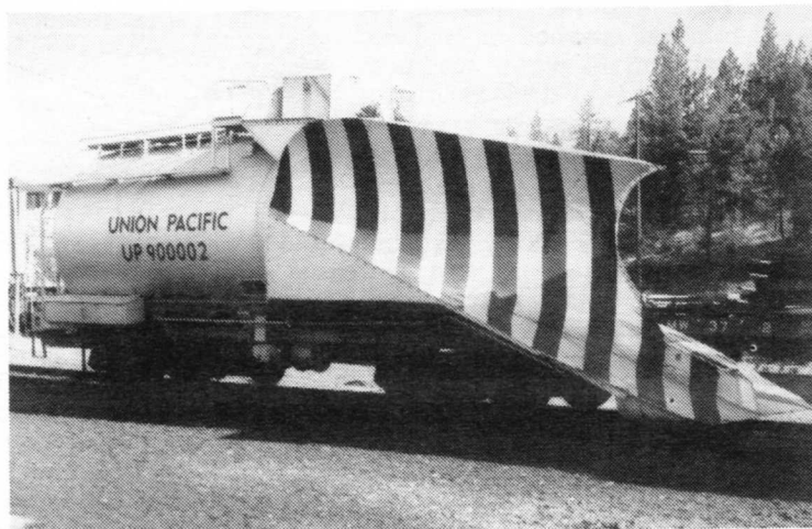
Snow Plow UP 900002 shown here at the museum with the side skirts removed from the front truck, and with roller bearings.
