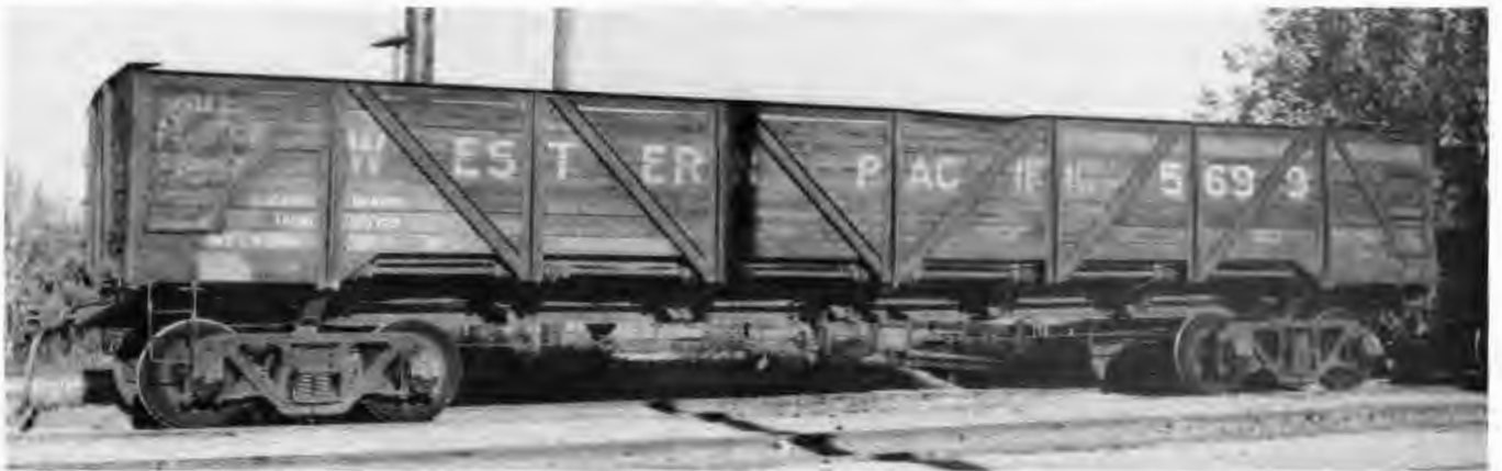
When photographed in 1939, this Western Pacific composite GS gon was exactly as built in 1918 except that Andrews trucks had replaced the original Arch Bar trucks. Note the shaft-and-chain mechanism for operating the drop bottom doors. WP owned 1,100 of these cars, numbered 4101-4500 and 5301-6000. Photo: W.C. Whittaker. No known decals.
