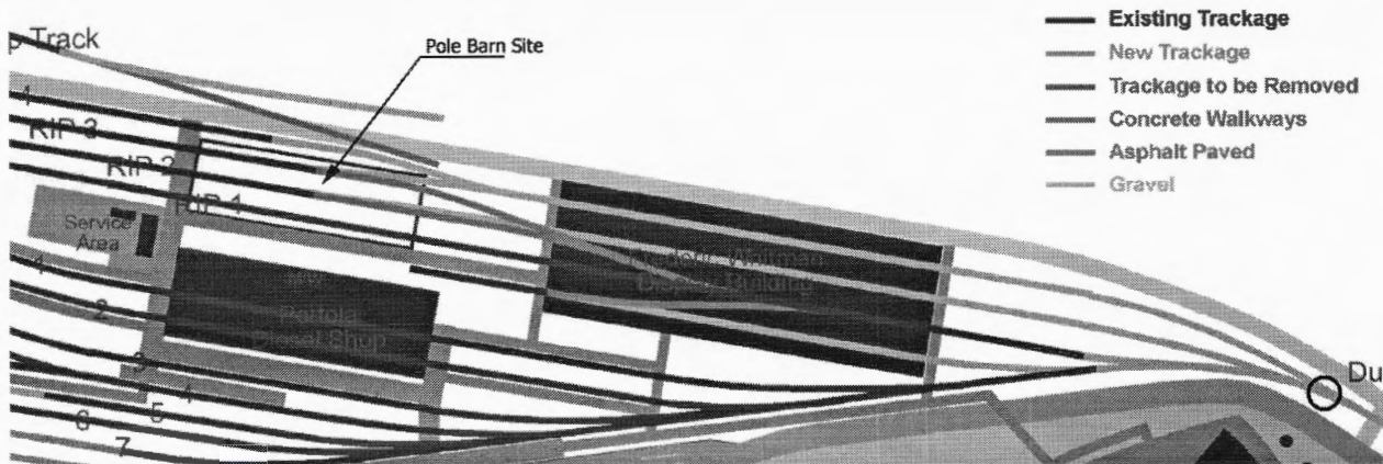
map shows reconfiguration of east end tracks and site of adopted pole barn plan
