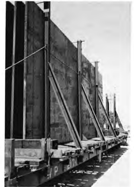
Metal bolsters prevent these horizontally-placed plates from sliding sideways.
