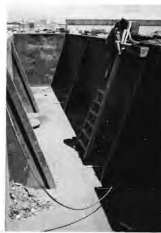
A member of WP's mechanical department attaches a wooden block to the inside of a gondola.
