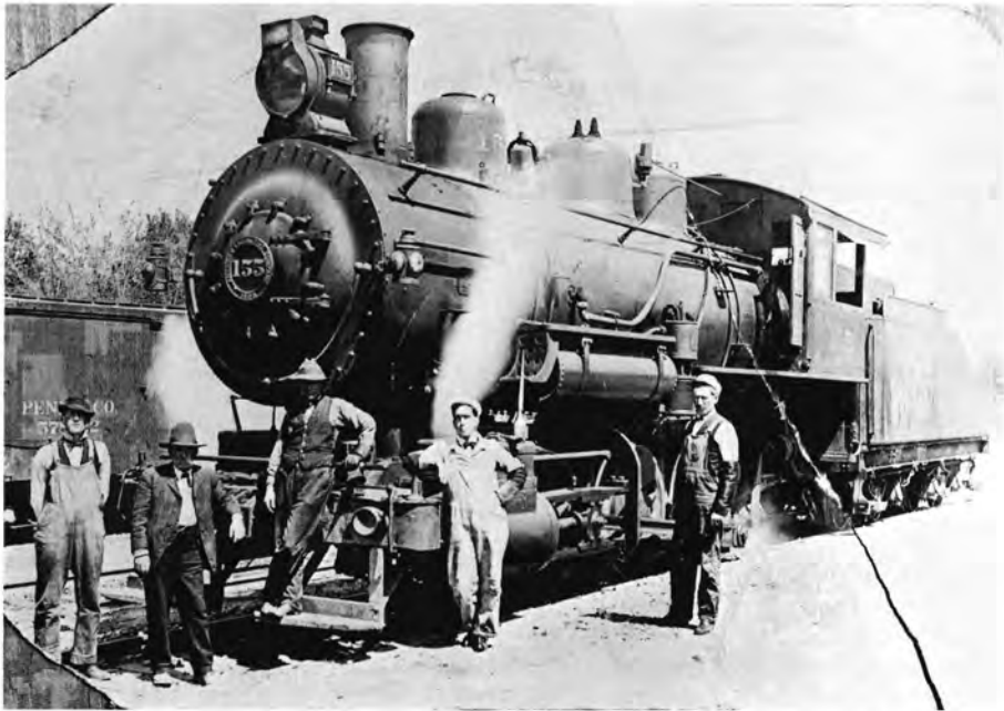
WP Locomotive #155 and crew pose for photo around 1910. This 0-6-0 class locomotive was built by the American Locomotive Works in 1909.
