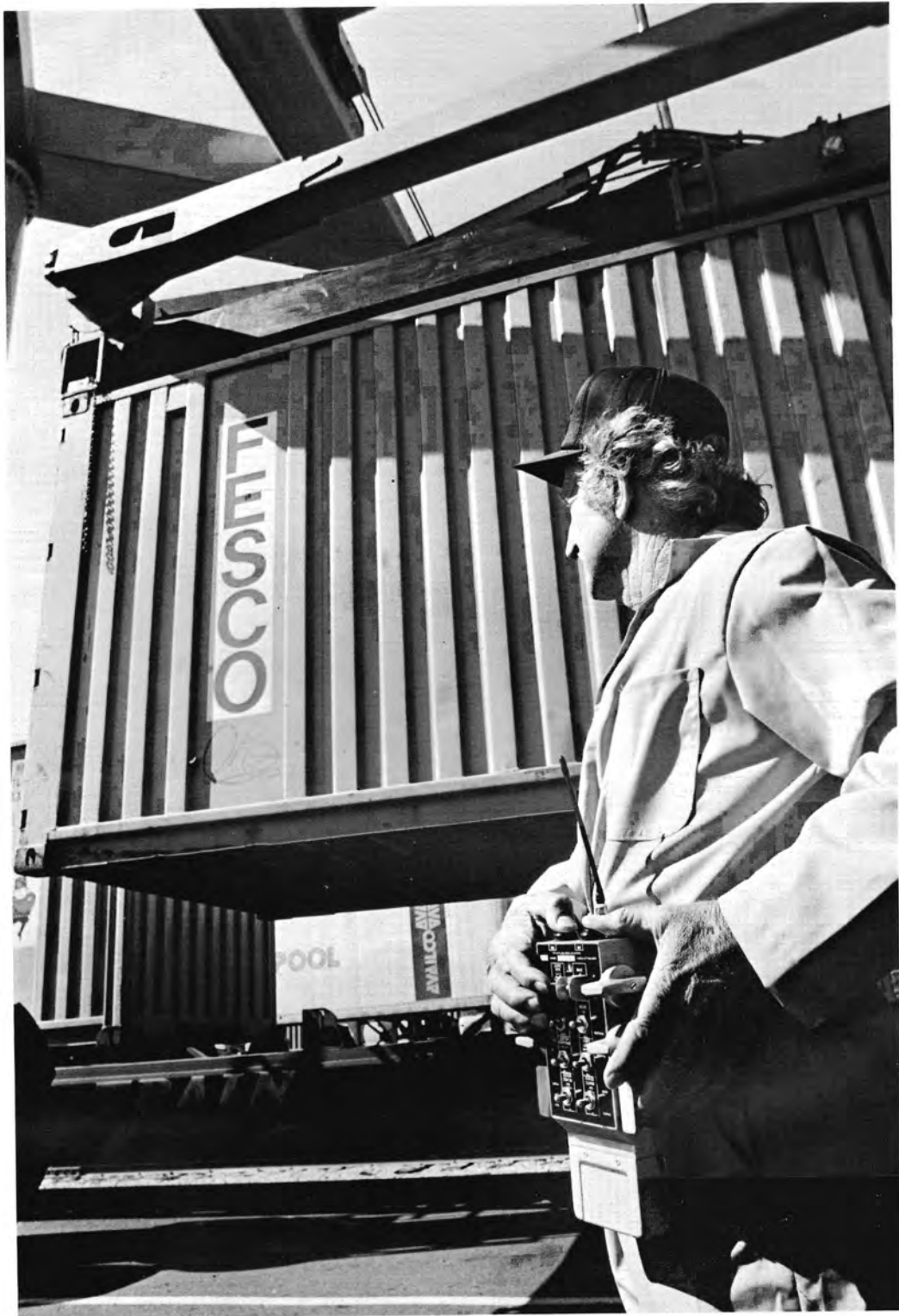
Radio control of 175,000 lb., 52-foot high Super Packer, by means of his belt-mounted modum, enables operator Curt Ellis to position himself at best vantage point for landing of container.
