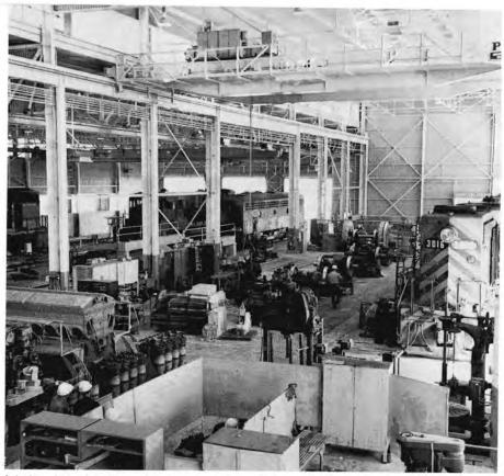
Interior view of portion of heavy repair bay shows 30-ton top running crane at top of picture. A 5-ton underhung crane system runs
