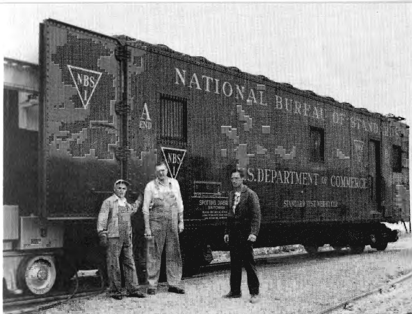
National Bureau of Standards' railroad car No. 1 carries a 7,500-lb. test car and test weights of various sizes. Left to right are E. D. Murphy, L. E. Lambrecht (NBS inspector), F. J. Hyatt.
