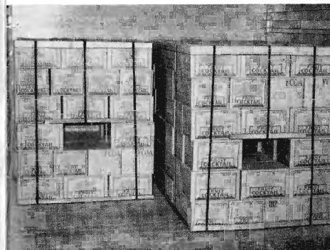
Right: Space between freight car doors can be easily filled; easily removed. Load rides well.
