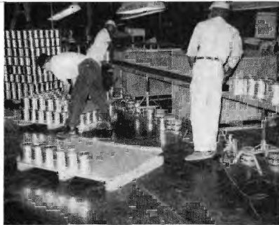
Uncased cans are placed on cardboard trays. Pallet is removed after unit is strapped.
