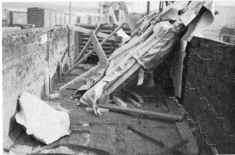
An illustration of the damage that can occur to a well-braced shipment of glass through rough and improper car handling. WP didn't lose the customer, but the claim was considerable.
