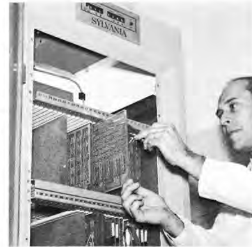
A Sylvania engineer changes modular circuit board in data conversion-transmission unit, which railroad personnel can plug in on-site if configuration changes necessary.
