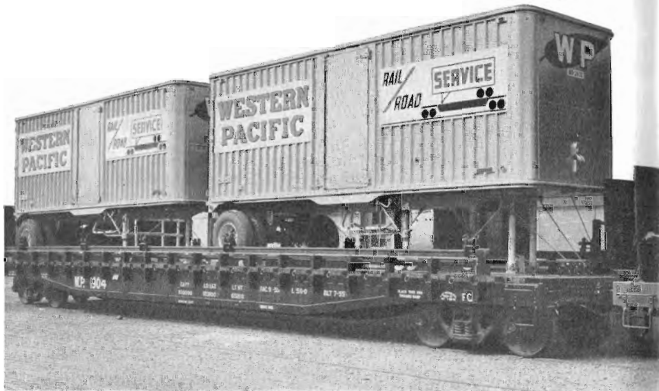
Trailer Train's 85-foot flatcars, like the one shown, are equipped with ACF type tie-down hitches, partially visible behind upright apron.
