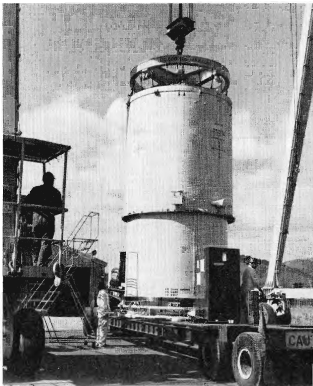
Shipping container is lowered over 40-ton solid-propellant rocket segment for protection during cross-country train trip to Cape Kennedy.
