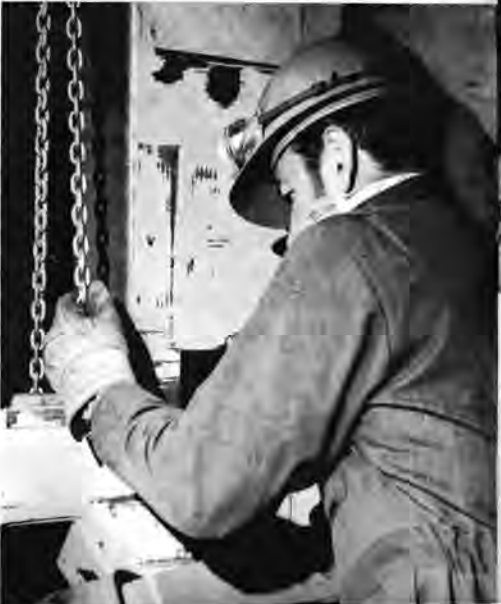
Raul wears heavy gloves for added protection and gets a firm grip when moving gates equipped with a chain and pulley action. He keeps his mind on what he's doing to avoid a hand injury should the chain or lever suddenly give way during movement of the heavy gate.
