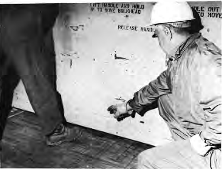
Frank Moreno points to danger area which can cause foot injury. When gates are pushed forward or pulled back they can swing from the top, raising the bottom edge from the floor. If a workman isn't careful, the gate can swing over the safety shoe cap and crush toes beneath area behind the cap.
