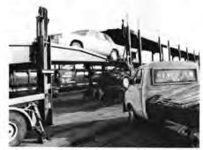
Commercial Carriers uses a mobile unit to carry bridge plates, jumper cables, gasoline, and other equipment to the multilevels. Photo by Andrew Partos, Berkeley, California.
