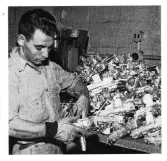
After the body has been die cast, burrs and excess metal are removed from the casting in cleaning operation.
