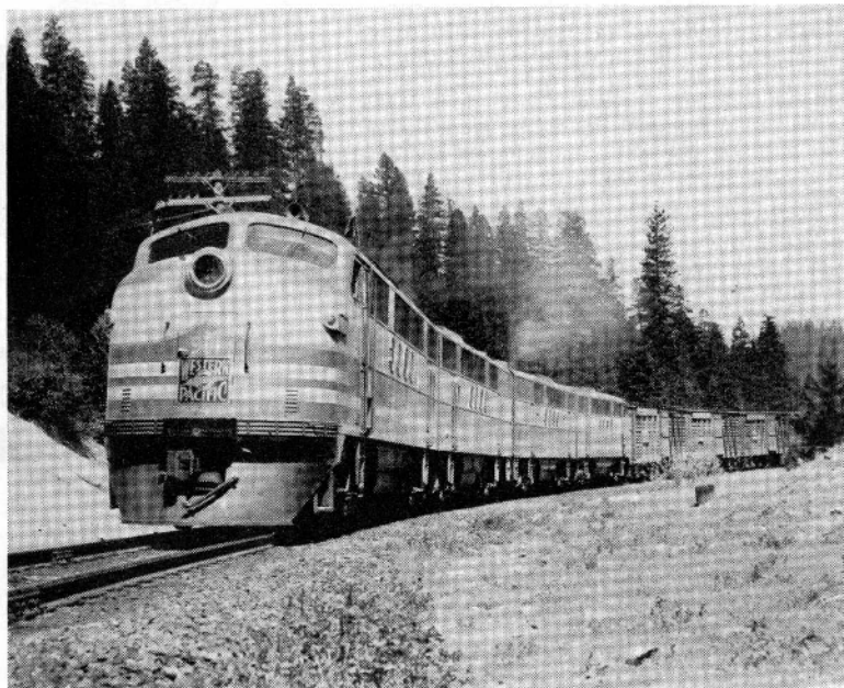
This photo shows a Western Pacific freight train, eastward bound, approaching Williams Loop (see text), in the upper part of the Feather River Canyon, California. The locomotive is a 5,400 h.p. Diesel-electric freight locomotive. Photographer Rudolph Haas of San Francisco was standing on the loop when he shot the picture.
