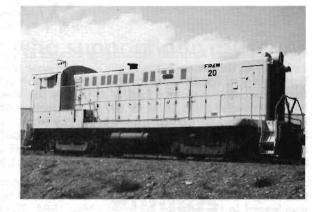
Baldwin-Lima-Hamilton Corp., model S-12, 1200 hp. Built June 1951, b/n 75053 ex-Oliver Mining 933 Purchased from USS/POSCO for resale by FRRS.
