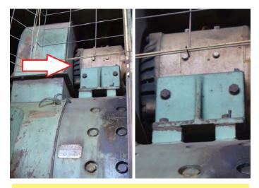
GP9 10KW Auxiliary Generator in SP 2873, sitting on top of main generator. - photos by Greq Elems
