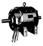
rotate the generator and start the engine. When the engine is running, it supplies mechanical power through shafts and couplings to directly drive two electrical generators. In addition to the main generator, there is an auxiliary generator that charges the storage battery and supplies low voltage direct current for the control, lighting, and main generator excitation circuits. The main generator supplies high voltage direct current to the traction motors for locomotive pulling power.
