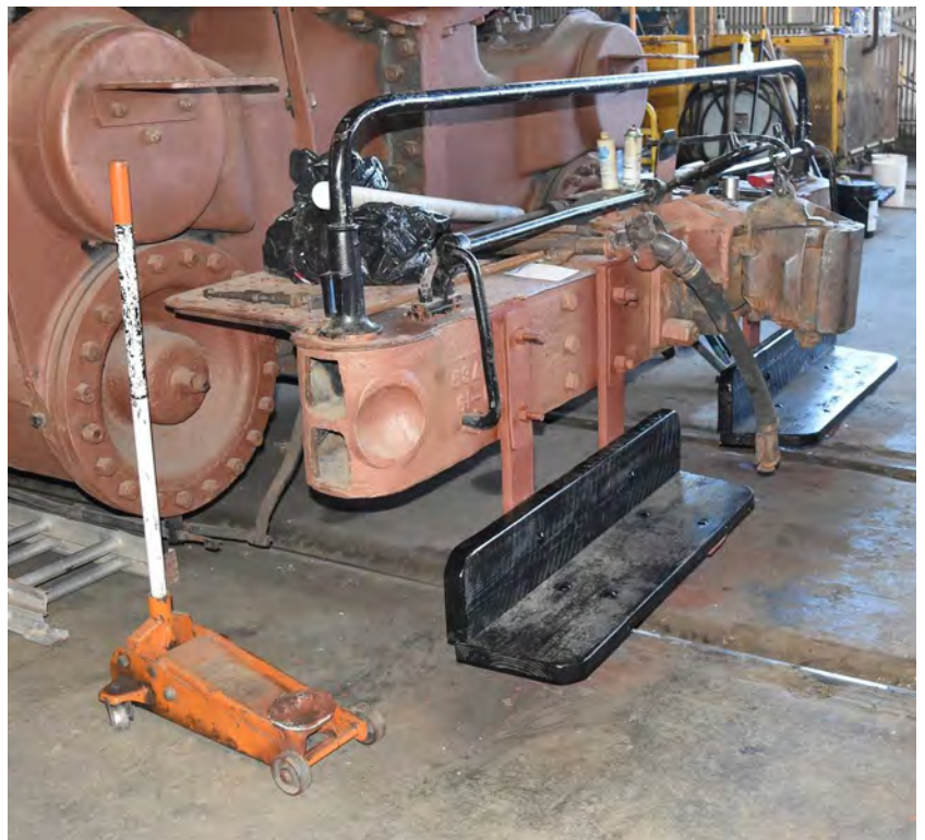
Bob Sims installed the front footboards on the WP 165 and Roger Stabler installed the brackets. 6/16/20
