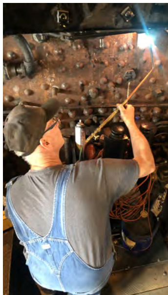
Roger heating the throttle support to fit the new throttle lever - photo by Mike Waters
