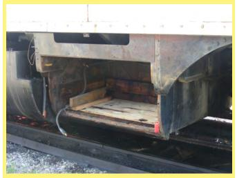
WP 917's right side battery box, prior to cleaning. Regular cleaning helps slow the corrosive effects of battery chemicals on the metal of the locomotive. The wood lining prevents terminals from inadvertantly touching the meal body. — David Elems Photo
