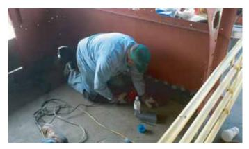
Dick Coudin drills holes for rivets at the base of the cab. - Chris Allan photo
