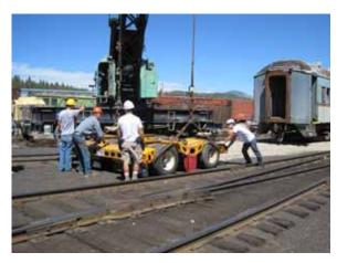
The crew confers on how to best position one of the trailer dollies. These trailers were positioned under the rear end of each car and allowed these long loads to be handled.
