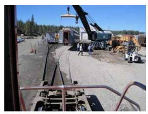
With one end in the air, the crew is ready for the lead trailer to be backed into place. The sub's truck is visible in the foreground through WP 608's handrails.
