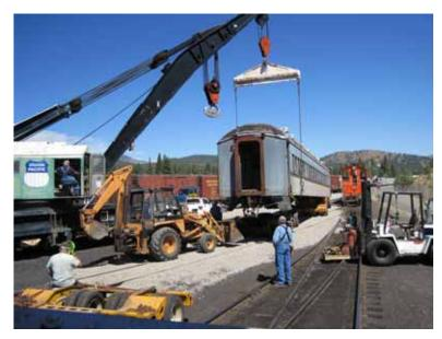
A good overview of just how complicated this could get. As WP derrick MW37 lifts, the backhoe is in place to pull the now released truckset. WP NW2u 608, in the background, pulled the first truckset to allow the lead trailer (the yellow visible under the far end of the car) to be backed into place. The following trailer, in the foreground, will be moved as soon as the truck is away. The big white forklift holds welding gear and other tools at the ready.
